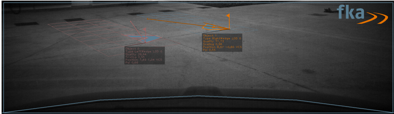
Figure 68: contour detection, one marker good quality, one marker poor quality, no cross validation
