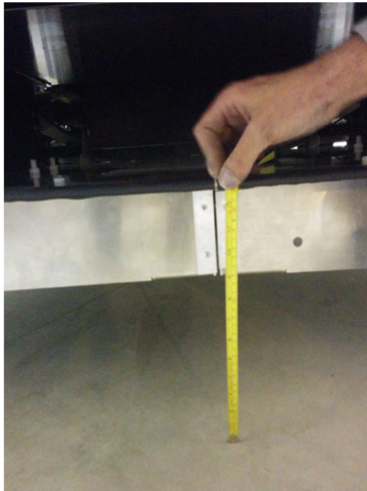
Figure 15 Adjusting the height of the secondary coils
