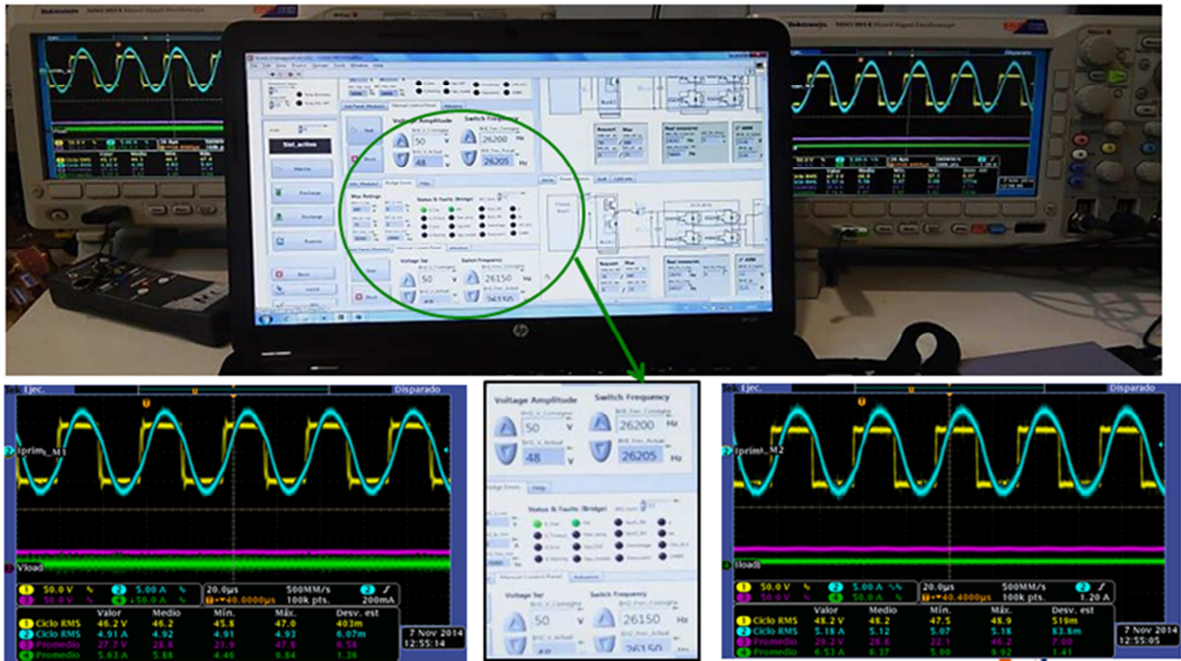
Figure 7 Adjusting frequency to compensate misalignment.
