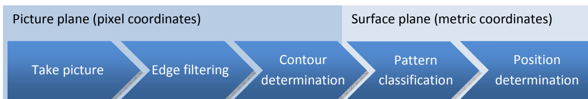
Figure 71: Process of position determination
