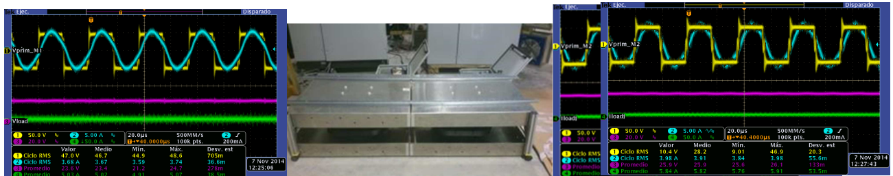
Figure 2 current (blue) and voltage (yellow) in both primary coils
