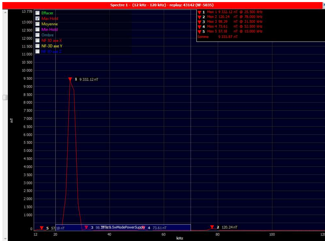
Figure 47: the highest value measurable is 9.3 \mu\text{T} , very close (20 cm) to the primary coil. This value is still lower than the ICNIRP value.
