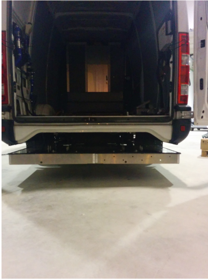
Figure 14 Secondary coils and EMI shielding installed in the Iveco Daily
