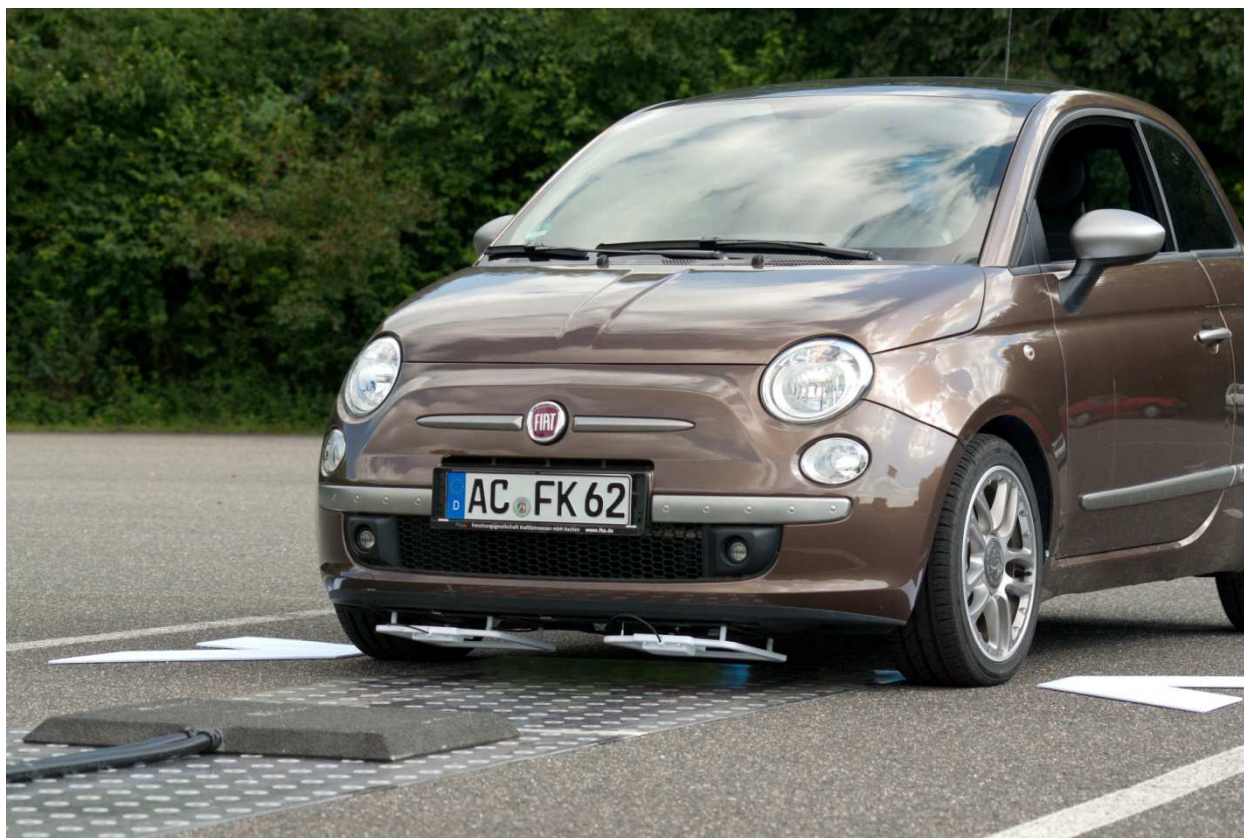
Figure 72: vehicle integration of RFID system (two antenna setup)
