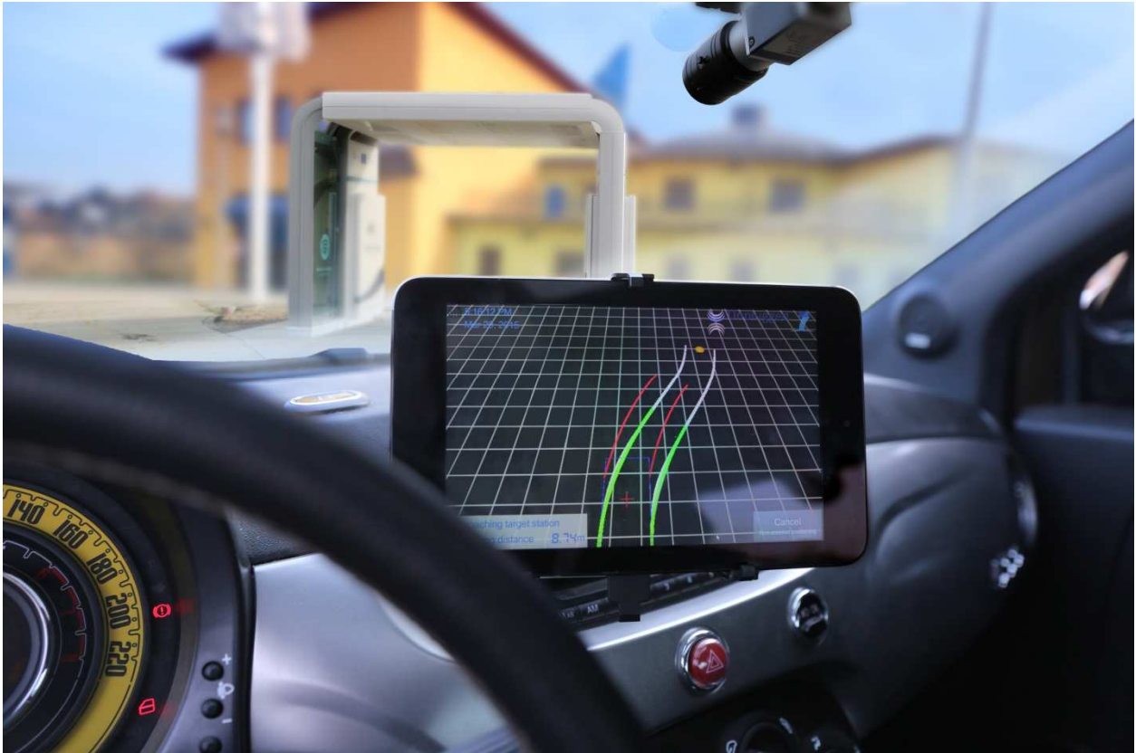
Figure 73: Human machine Interface showing a planned trajectory
