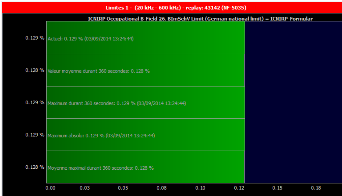
Figure 59. Maximal value obtained during all the measurements. In that case, the primary coil was misaligned of 20 cm in the X direction.
